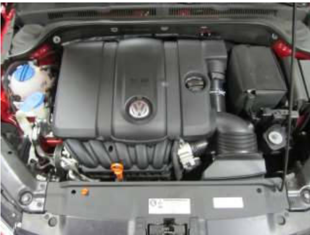
Factory air box system installed
