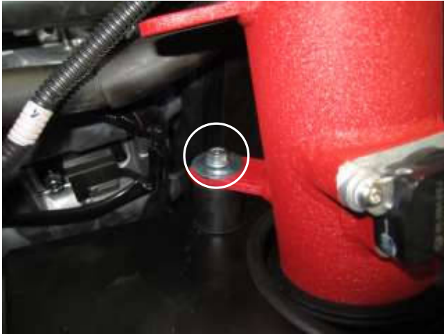
l. Align the bracket with the rubber mount and tighten the washer (08160) and nut (444.460.04).
