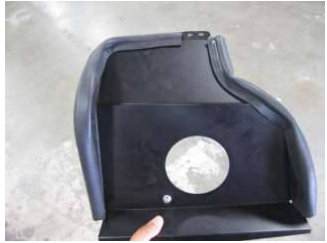
d. Install the supplied edge trims (102494 & 8-4013) onto the outer part of the heat shield.
