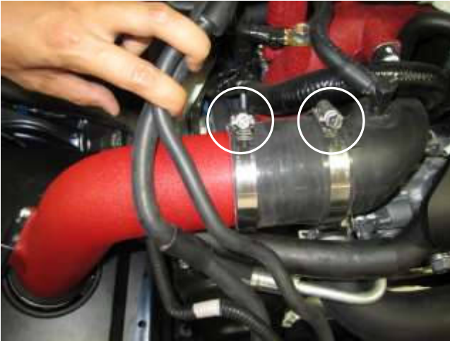
k. Install the supplied coupler (5-275) and tighten the two hose clamps (9444) onto the AEM intake tube and compressor inlet tube.
