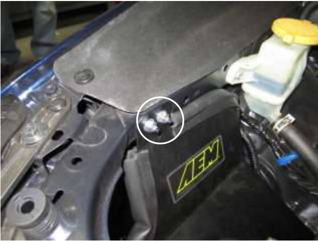
i. Re-install the nuts that were removed 2c) and tighten.
