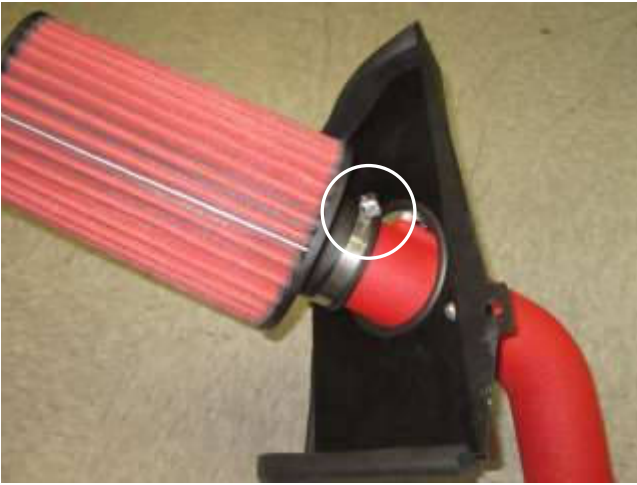
g. Install the AEM filter onto the AEM intake tube through the heat shield and tighten the hose clamp (9448)
