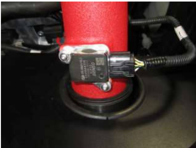
n. Plug in the mass air flow sensor connector that was detached in 2b.
