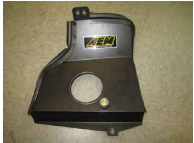
f. Completed heat shield assembly.
