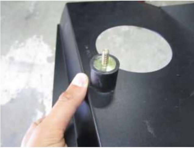
c. Install the rubber mount (1228599) onto the heat shield and secure with nut (444.460.04) on the back side.
