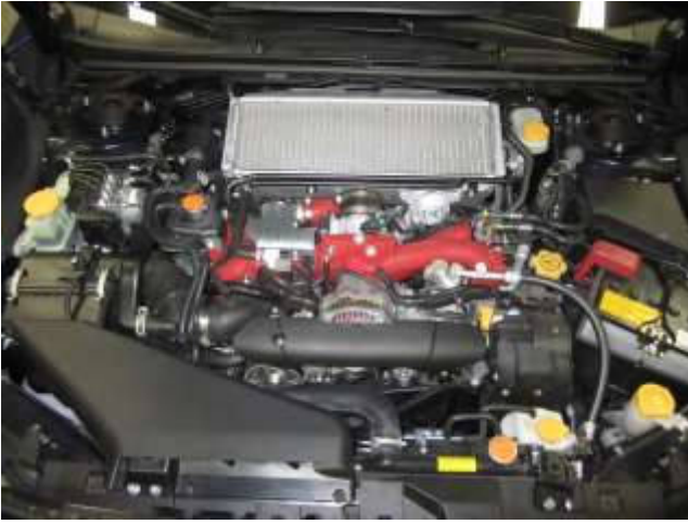
Stock Intake Installed.
