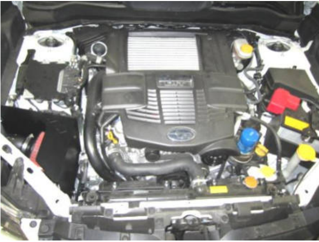
k. AEM intake system installed.
