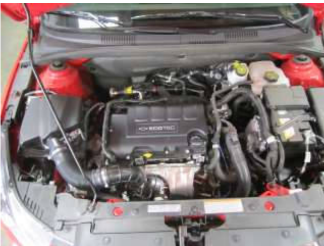
STOCK INTAKE INSTALLED
