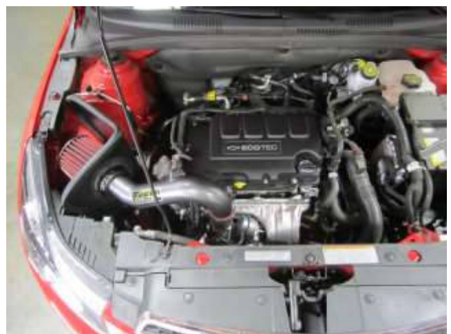
AEM INTAKE INSTALLED
