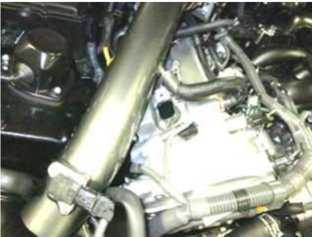
i. Reconnect the PCV hose to the AEM tube provision and the harness to the MAF sensor.
