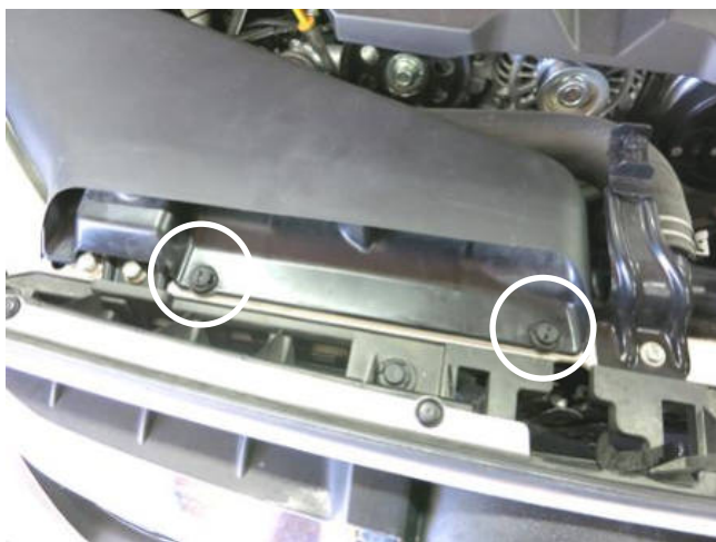
a. Remove the scoop and the two clips from the vehicle. The scoop will not be reinstalled but do not discard.
