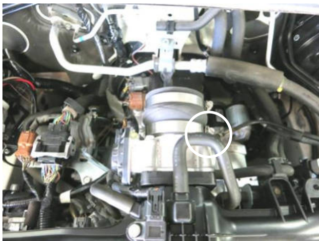
c. Install the provided hose and hose clamps onto the throttle body. Tighten the hose clamp closest to the throttle body now.
