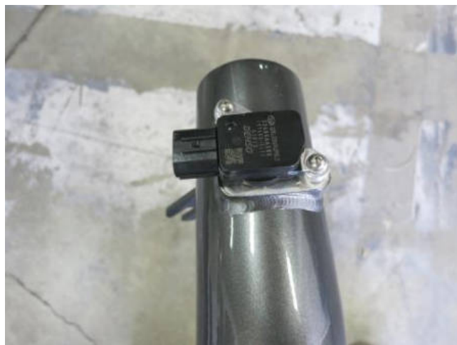
d. Install the MAF sensor that was removed in step 2h. and secure with the provided Allen head bolts.
