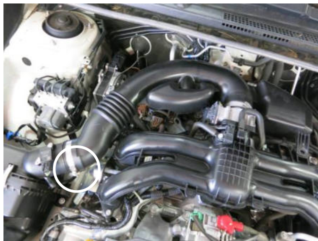
d. Loosen the hose clamp at the air box and remove the stock intake tube from the vehicle.
