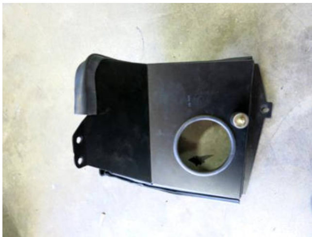
a. Install the edge trim and rubber mount onto the AEM heat shield according to the parts diagram on pg. 2.
