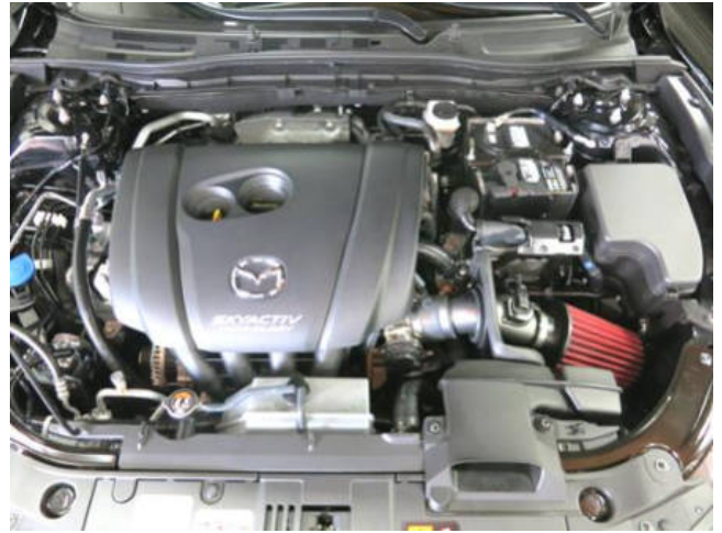
p. Finished installation of AEM Intake System.
