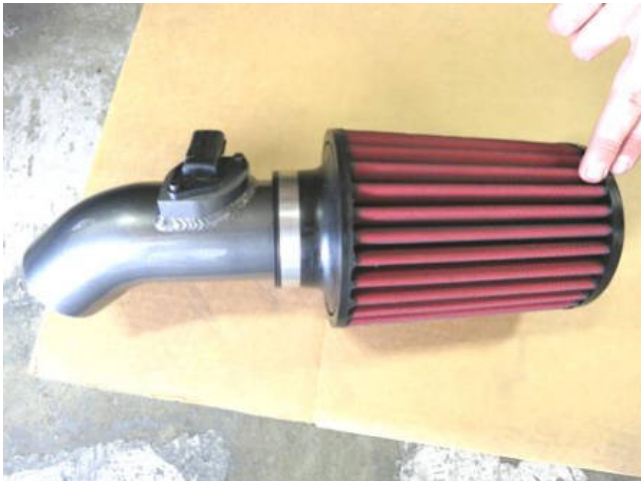
j. Loosely install the AEM air filter onto the intake tube.
