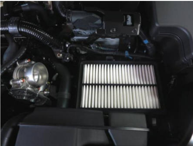
g. Remove the air box lid along with the air inlet hose.
