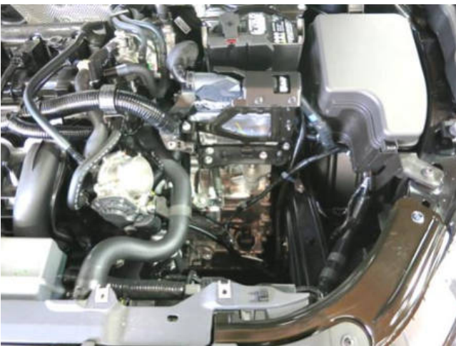
i. Gently remove factory lower air box and factory cold air inlet scoop.
