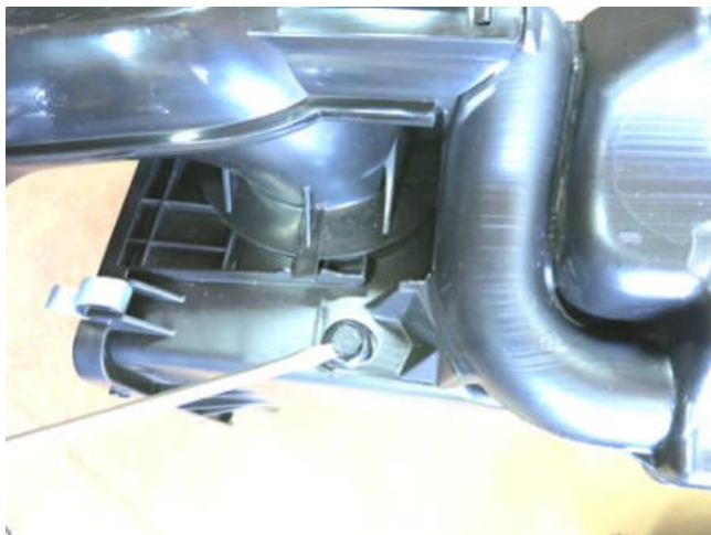
a. Unclip the two plastic retainers securing the cold air inlet scoop to the factory air box.
