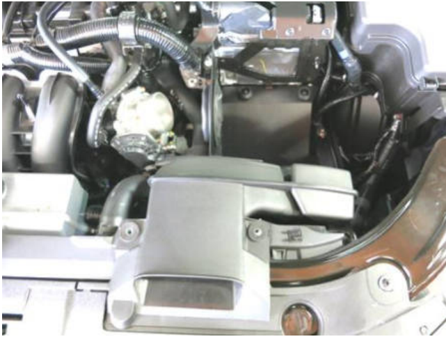
f. Insert the factory cold air scoop into the AEM heat shield and install assembly using factory grommets.
