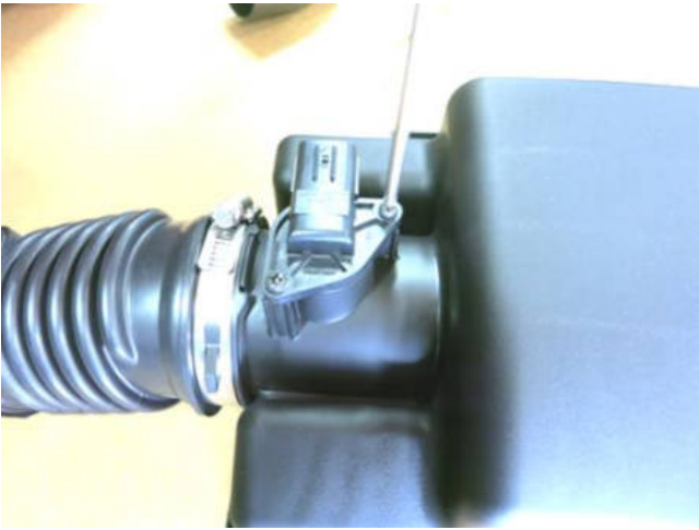
g. Remove MAF sensor from the factory air box using a small Philips head screw driver.
