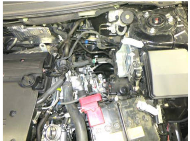
h. Remove the factory intake from the vehicle. Note: Do not discard any of your stock equipment.
