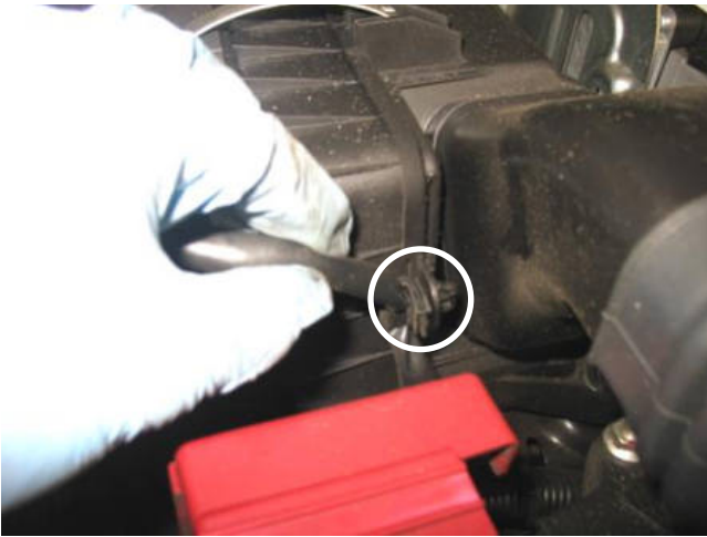
e. Detach the MAF sensor wiring clip from air box.
