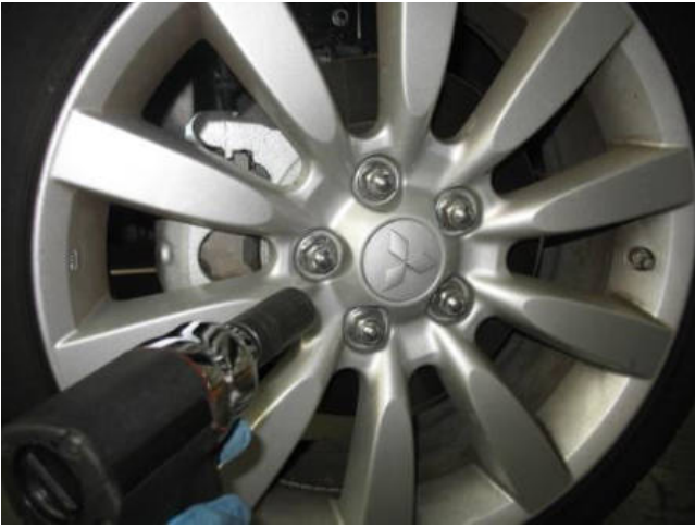
k. Remove the front drivers side wheel with a 21mm socket. This will be re-installed in step 3o.
