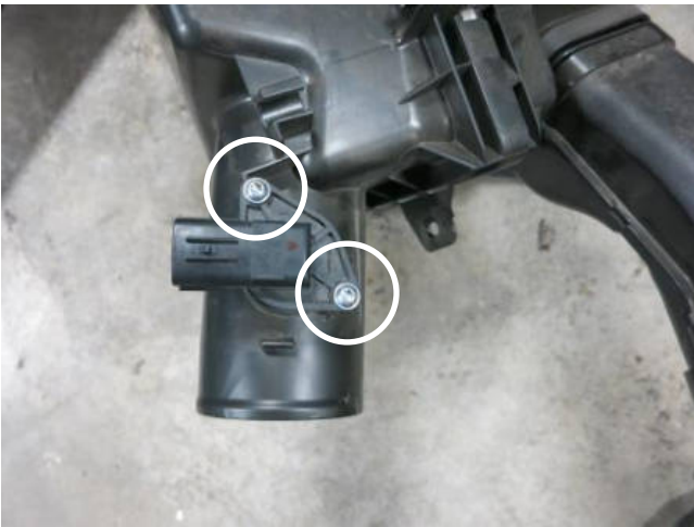
m. Remove the MAF sensor with the supplied T20 L-Key. This will be re-used in step 3d.
