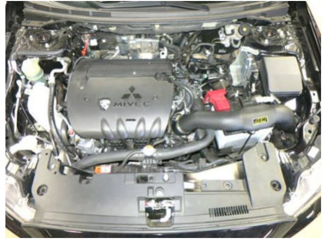
AEM INTAKE INSTALLED
