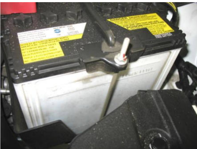
i. Remove the factory J-hook on the front side of the battery tie down. Push the battery toward the back of the vehicle. The nut will be re-used in step 3a.
