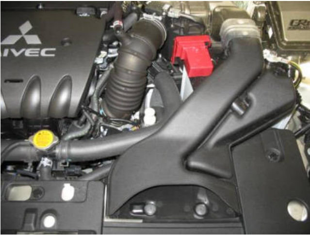
STOCK INTAKE INSTALLED
