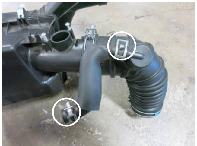
n. Remove the two springs clamps circled. These will be reused in step 3m.
