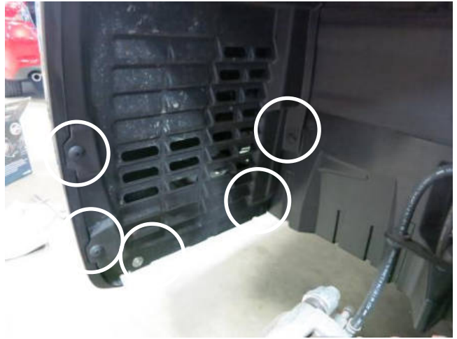
l. Remove the driver side fender well liner, it is secured to the wheel well with plastic clips and a 10mm hex bolt. This will be re-installed in step 3n.
