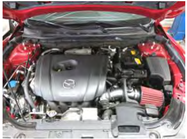
p. Finished installation of AEM Intake System.
