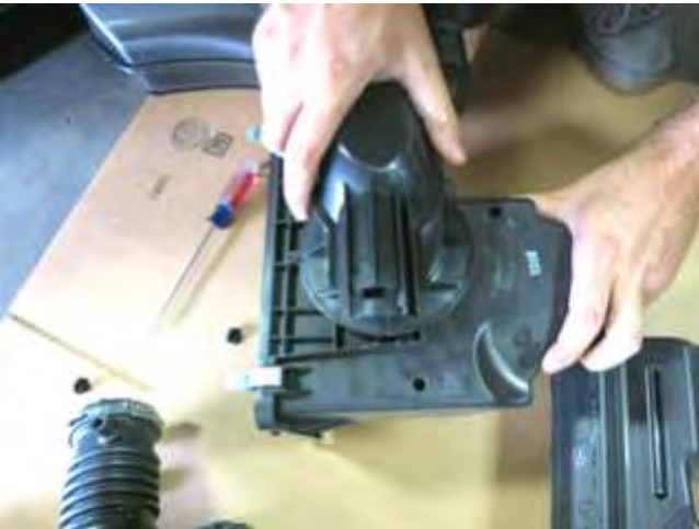
c. Separate the cold air scoop from the lower air box.
