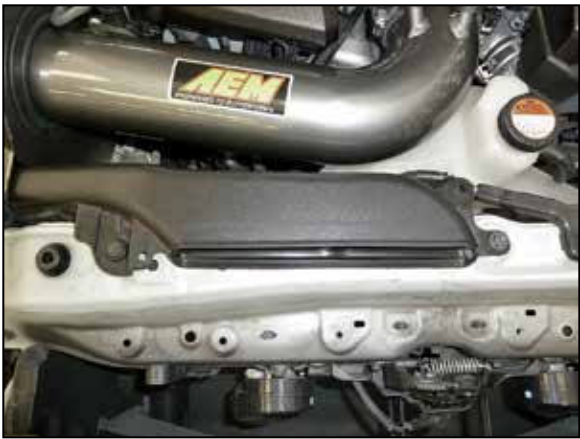
19. Reinstall the fresh air intake duct and secure with the factory Hardware.
