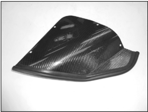
21. Install the remaining edge trim onto the Carbon Fiber filter lid.
