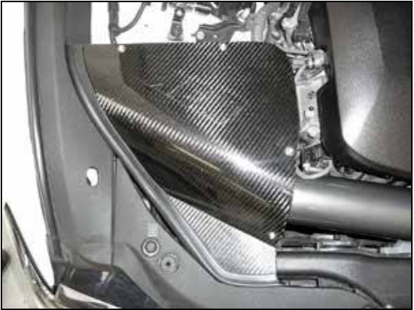
22. Install the carbon fiber lid assembly onto the heat shield and secure with the provided hardware.
