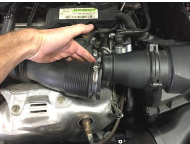
c. Loosen hose clamp at the factory airbox connection and remove as shown.
