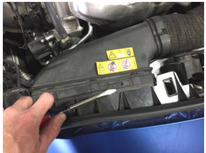
b. Release factory inlet duct with a small flat blade as shown and pull downward to fully disconnect.
