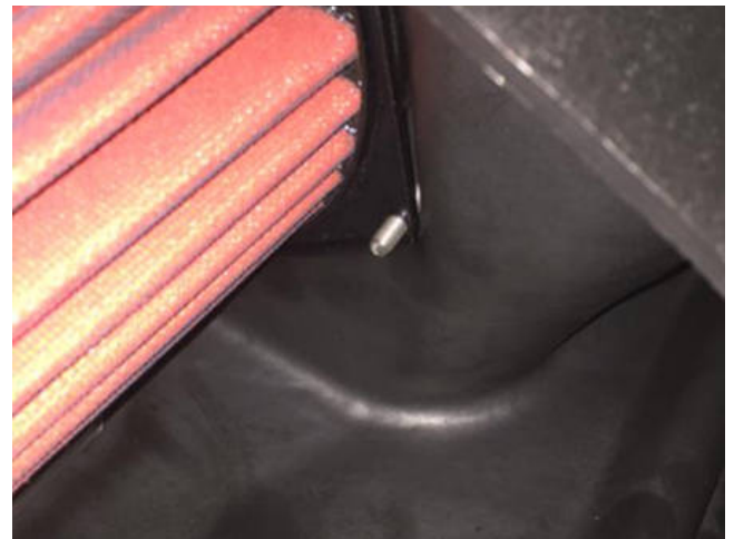
d. Tighten all three mounting screws with uniform torque until about 12mm of the fastener protrudes through the retainer ring.
