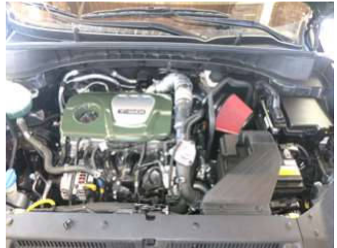
AEM INTAKE INSTALLED
