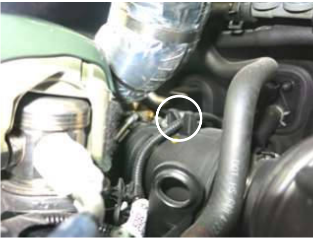
g. Remove the wiring harness loom from the clip in the stock intake tube and remove the stock intake tube from the vehicle.
