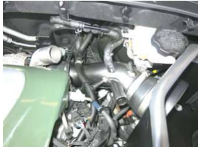
l. Push the heat shield down to secure the stand-off into the grommet in the vehicle while aligning the intake tube with the coupler.
