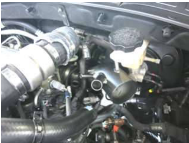
j. Install the AEM intake tube into the coupler at the turbo compressor. Note: Soapy water will help installation and adjustment.
