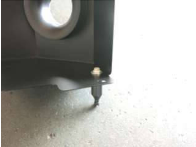
d. Install the stand-off and provided hardware onto the heat shield. You will install it on the inside hole.
