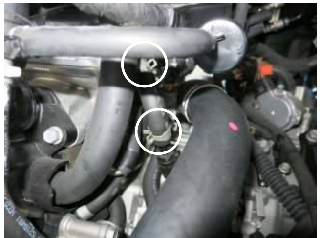
j. Follow the hard line from the previous step to the "T" fitting. Remove the short vent line and spring clamps from the hard line to the "T" fitting. The spring clamps will be reused in step 3g & 3i.
