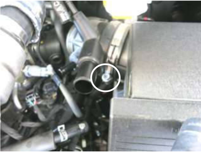
e. Loosen the hose clamp at the stock air box. Then remove the stock air box from the vehicle.
