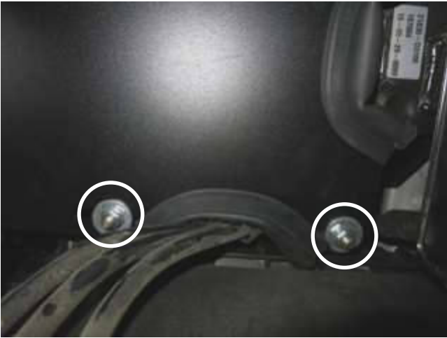
k. Install the completed heat shield into the vehicle aligning the slots in the shield to the previously installed studs. Install the washers/nuts and tighten.
