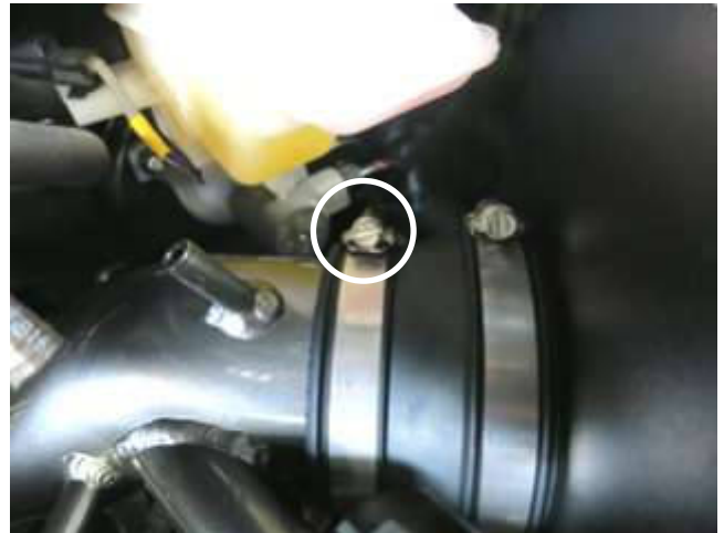
n. Tighten the hose clamp on the coupler at the heat shield.
