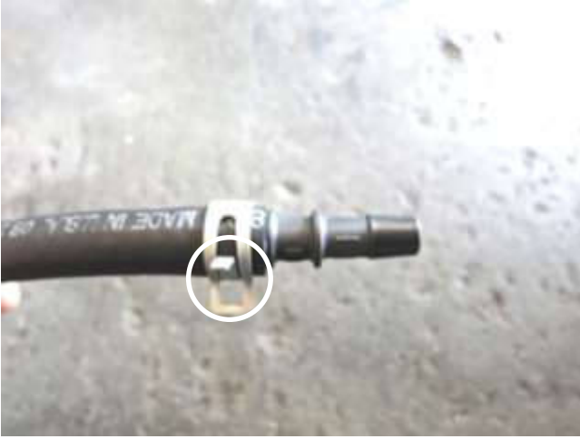
g. Using the providing hose, install the union into one end and secure with a spring clamp removed in step 2j.
