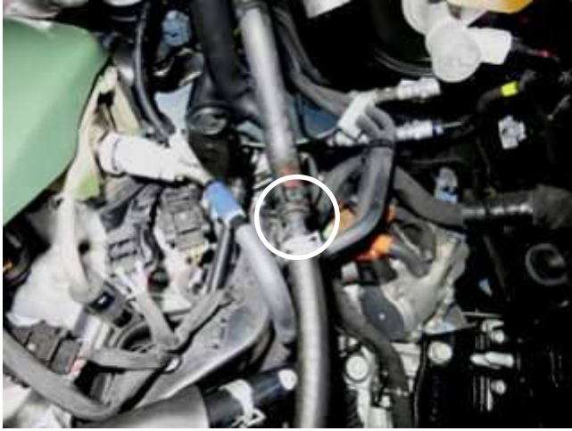
h. Connect the previously assembled hose to the EVAP vent line that was disconnected in step 2i, and secure with the spring clamp.
