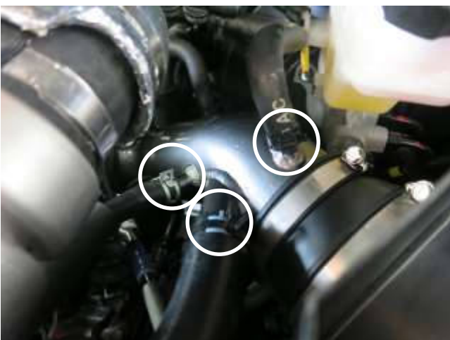
o. Install the vent hoses and spring clamps that were removed in step 2c.
