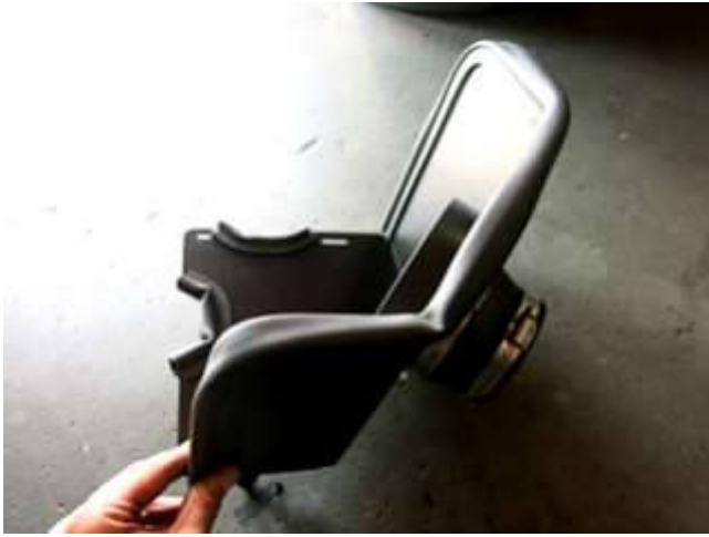
f. Install the provided edge trim onto the completed heat shield. Note: Some trimming may be necessary.
