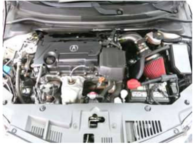
AEM INTAKE INSTALLED
