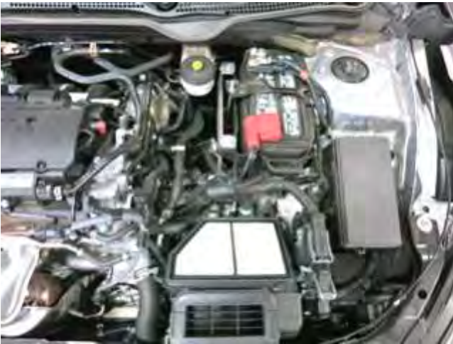
g. Remove the upper air box with the intake arm.
