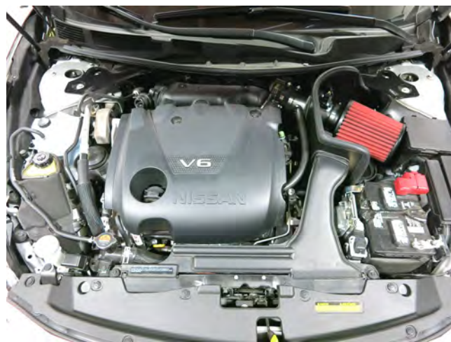
AEM INTAKE INSTALLED
