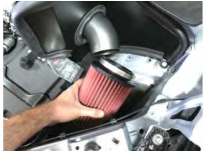
l. Position the AEM air filter into the engine bay as shown and maneuver it onto the AEM intake tube.
