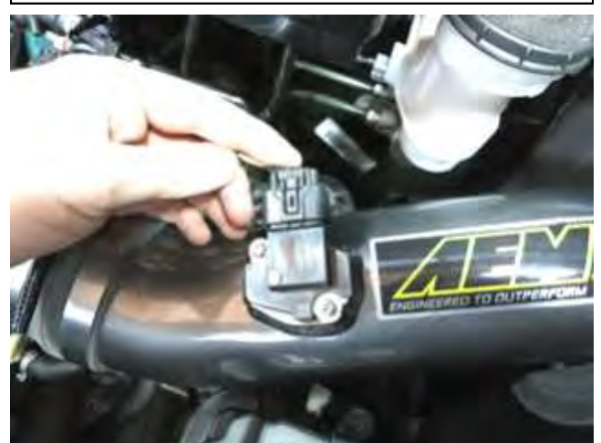
n. Attach the sensor connector to the MAF sensor.
