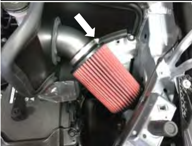
m. Tighten the hose clamp on the air filter to 30in-lbs.
