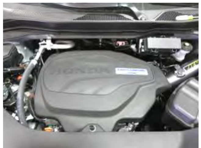
p. Reinstall the plastic core support cover by sliding it under the hood latch into position and gently pressing down, snapping it into place from left to right. Then, reinstall the plastic engine cover by aligning the rubber grommets with their posts and gently pressing down.
