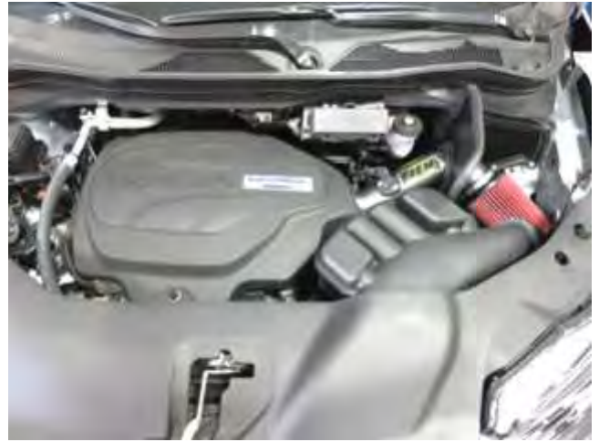
AEM INTAKE INSTALLED
