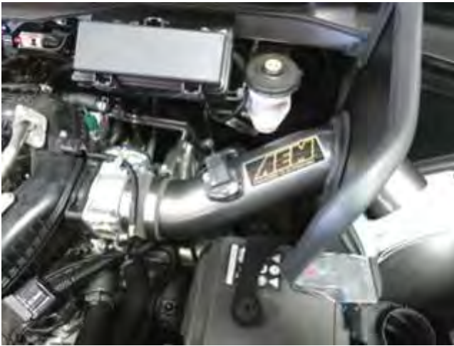
k. Install the vent hose onto the nipple on the AEM intake tube and insert the AEM intake tube into the coupler.
