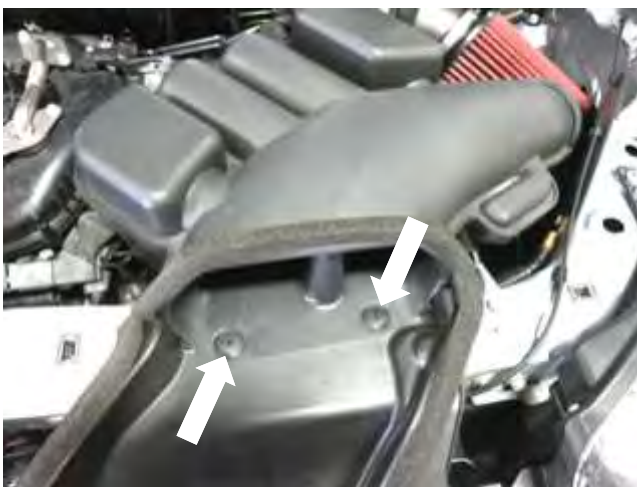
o. Reinstall the cold air duct and plastic pop-outs removed in step 2g. Note: Use care to not drop the clips as they are easily lost in the core support area. Position the AEM intake for best fit and tighten the hose clamp at the coupler to 30in-lbs at this time.
