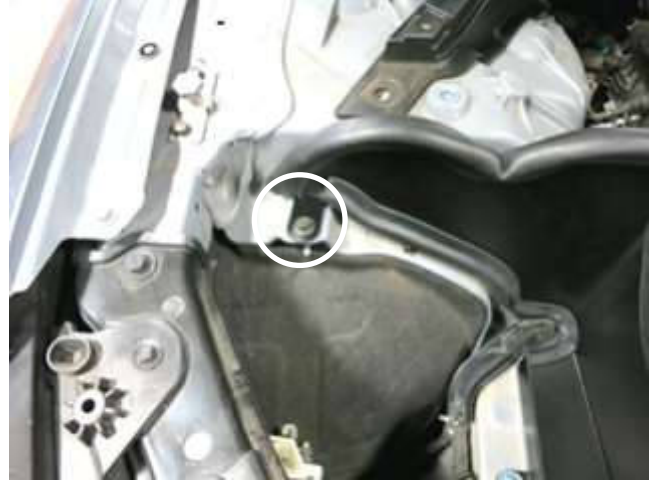
f. Using a bolt from step 2h, secure the heat shield to the vehicle.
