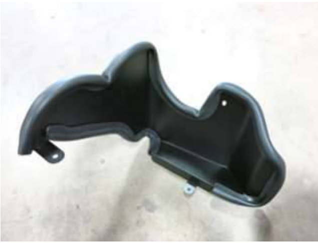
c. Install the provided edge trim around the AEM heat shield as shown. Note: Cutting the trim to fit will be necessary.
