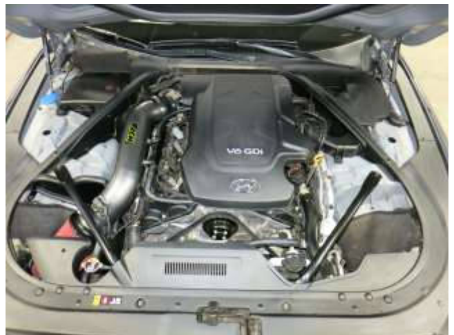
AEM INTAKE INSTALLED
