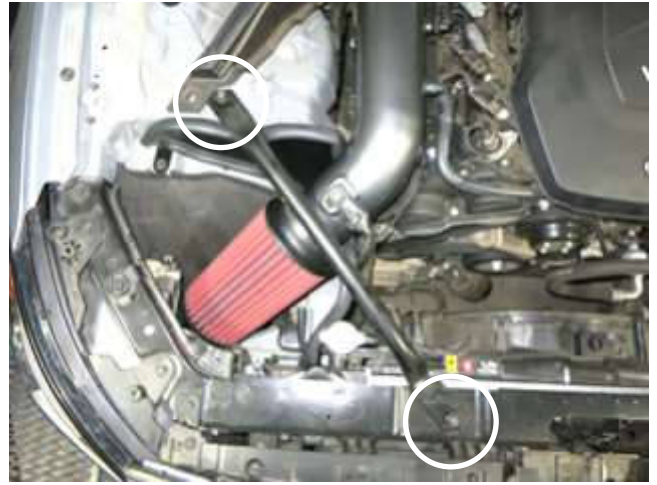
p. Reinstall the brace and bolts onto the vehicle and tighten to 3.6 ft-lbs.
