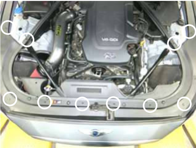
q. Reinstall the engine bay cover into the vehicle and secure with the clips removed in step 2a. Note: You will only use 12 of the clips (not all pictured)
