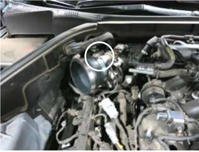
g. Install the provided coupler onto the throttle body, tightening the hose clamp closest to the throttle body to 30 in-lbs.
