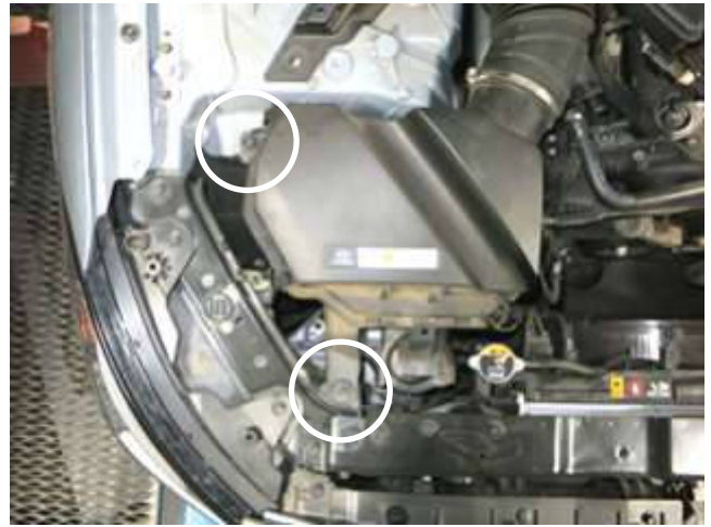
h. Remove the two bolts securing the air box to the vehicle. Note: One of these bolts will be reused in step 3f.
