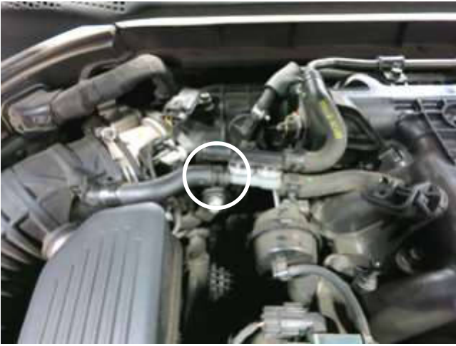
e. Release the tension on the spring clamp, and remove the hose from the 2-way check valve.
