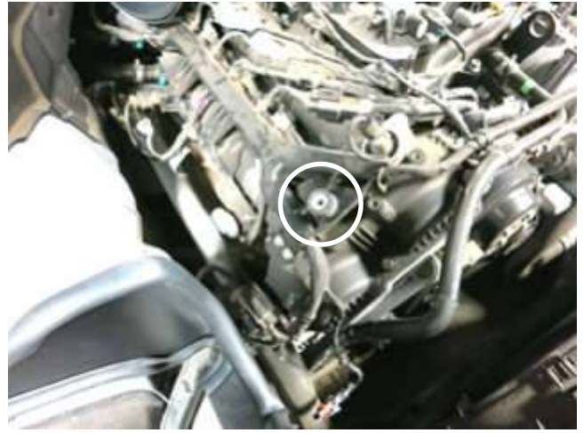
h. Install the provided rubber mount onto the passenger valve cover where the original bolt was removed in step 2k.
