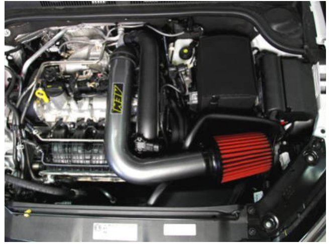
AEM INTAKE INSTALLED
