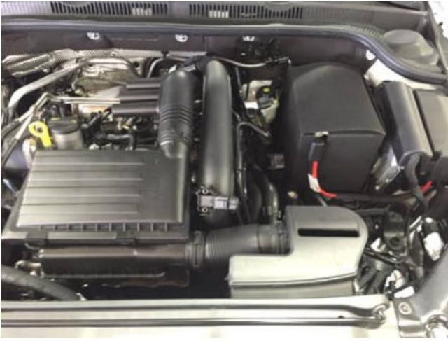
STOCK INTAKE INSTALLED
