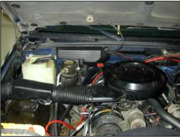
Factory air box system installed
