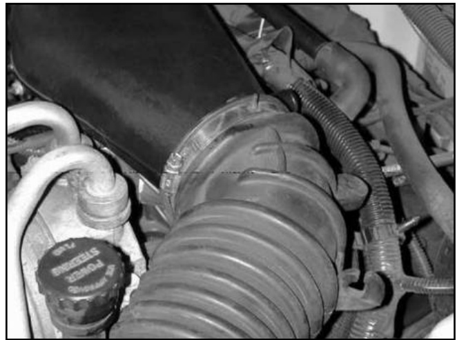
d. Loosen the hose clamp securing the stock intake tube to the plastic throttle body adapter. Remove the entire air box lid / MAF sensor / intake tube assembly from the vehicle.
