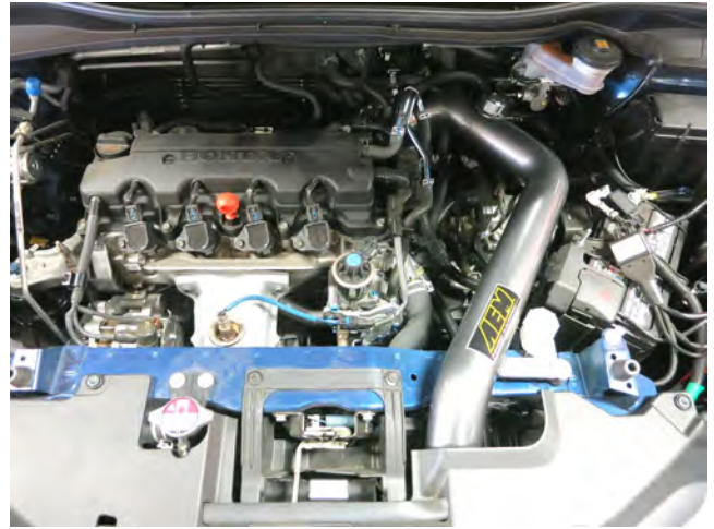
AEM INTAKE INSTALLED
