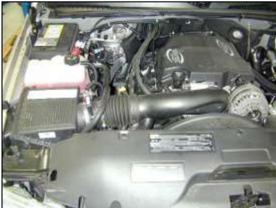
a. Factory airbox system installed.
