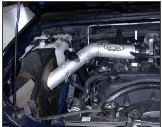
AEM® intake system installed
