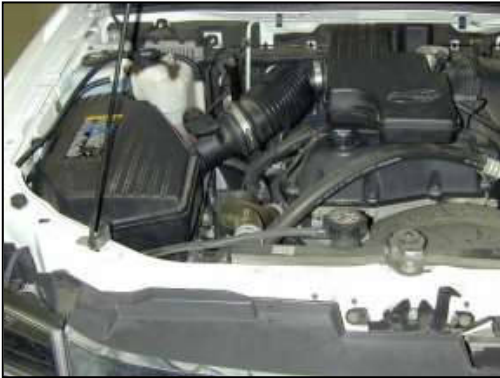
a. Factory airbox system installed.
