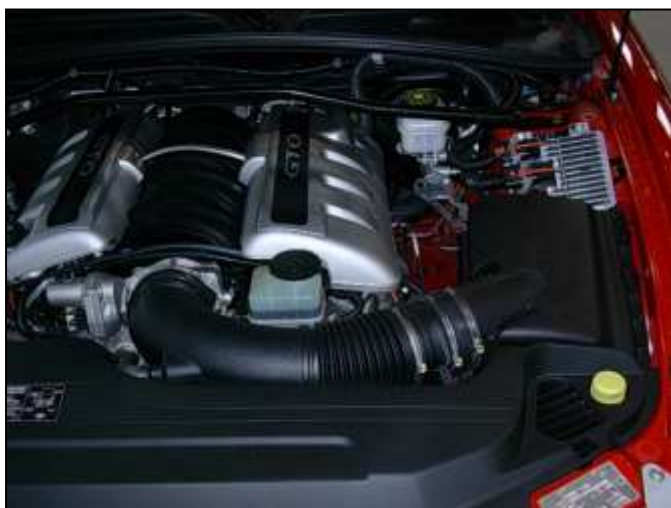
Factory air box system installed
