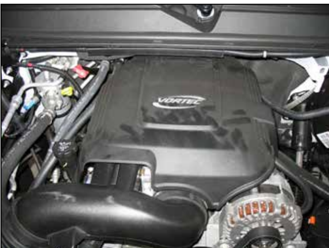
Factory airbox system installed
