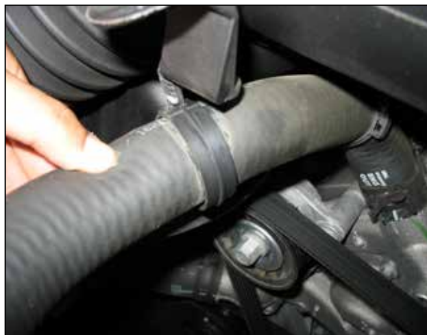
d. Pull the plastic radiator hose tree mount out of the stock intake tube holder.
