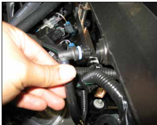
b. Pull out the breather hose out of the resonating chamber in the stock intake system.
