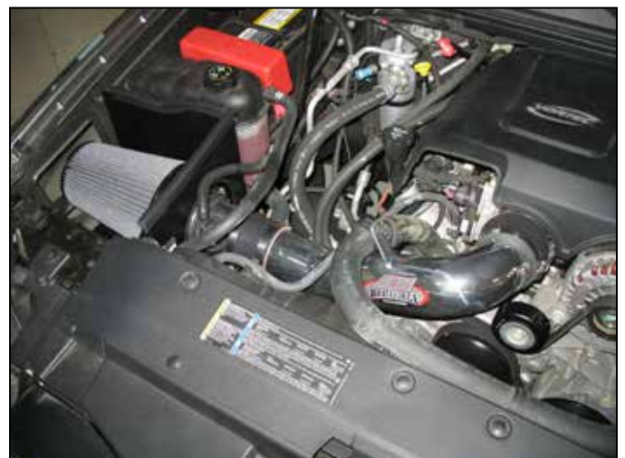
AEM® intake system installed
