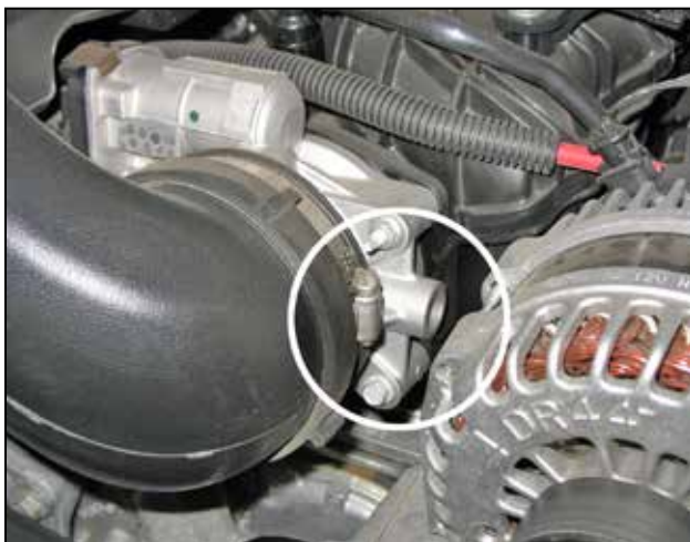
c. Loosen the hose clamp located at the throttle body.
