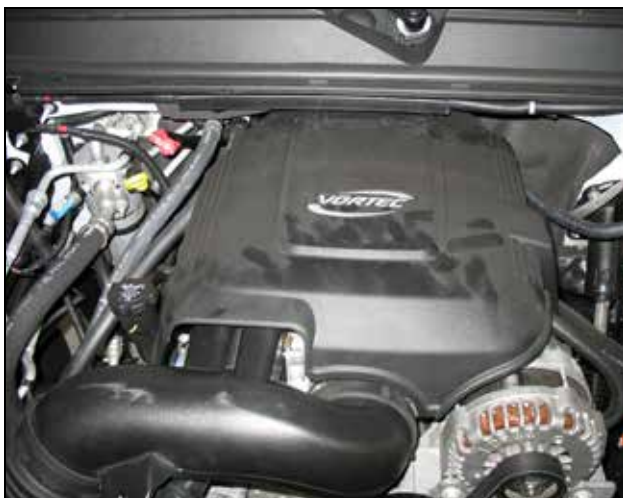
a. Stock airbox system. Pull engine cover off.
