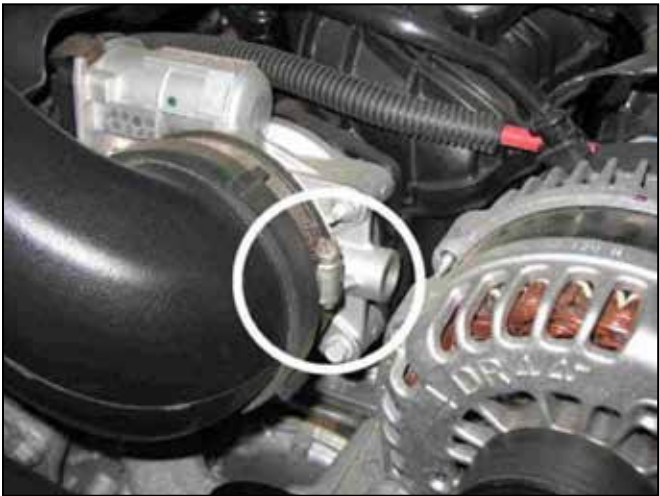
c. Loosen the hose clamp located at the throttle body.
