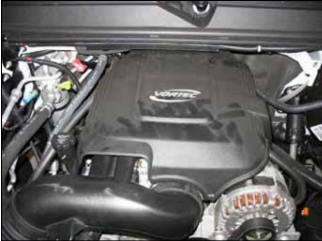
a. Stock air system installed system. Pull engine cover off.
