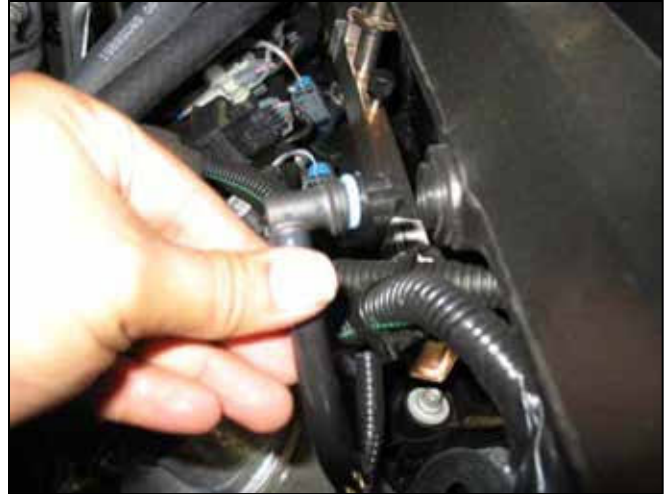
b. Pull out the breather hose out of the resonating chamber in the stock air box system.
