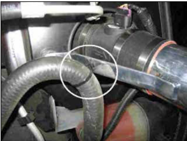
n. Insert tree mount into intake pipe bracket, secure radiator overflow hose to tree mount.
