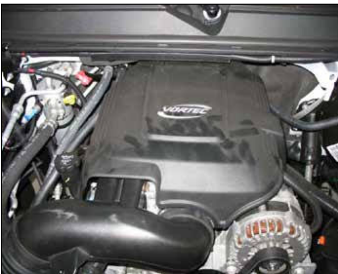
Factory air box system installed
