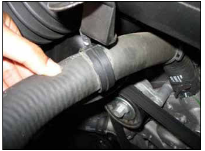
d. Pull the plastic radiator hose tree mount out of the stock intake tube holder.
