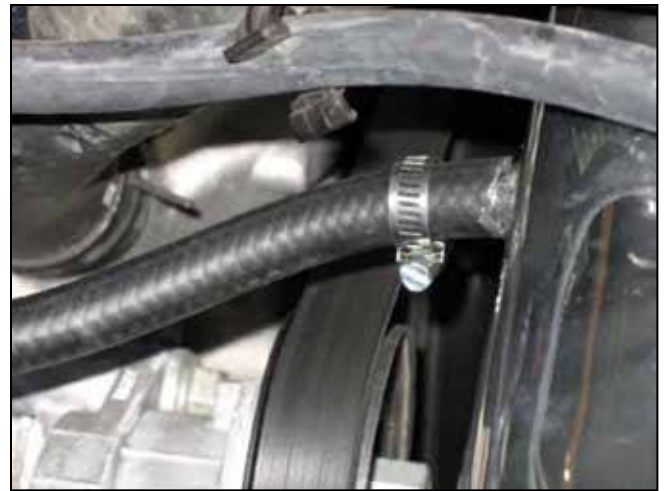
m. Secure the breather hose to the nipple on the intake pipe.
