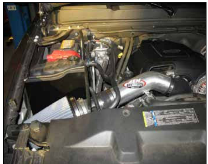
AEM® intake system installed
