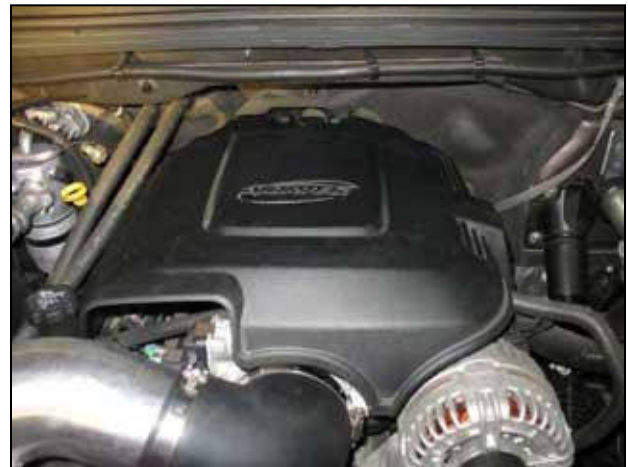
o. Reinstall the engine cover.
