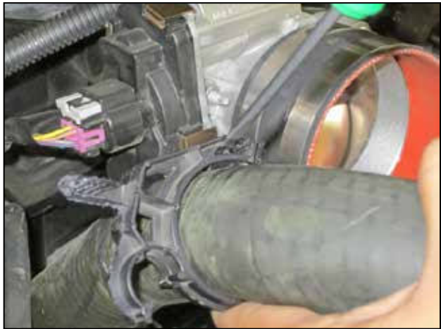
o. Flip the plastic clip around and position it on the upper radiator hose as shown.
