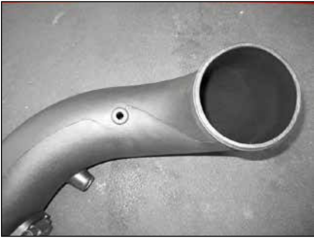
j. Install the grommet in the intake tube.
