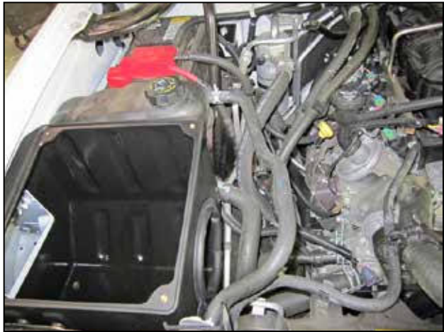
m. Replace the overflow tank in its original location and fasten it with the factory nut and bolt that were removed in step 2k.
