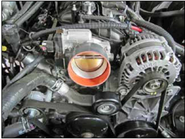
k. Install the coupler onto the throttle body.
