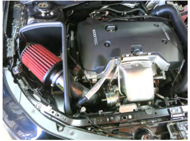
AEM INTAKE INSTALLED
