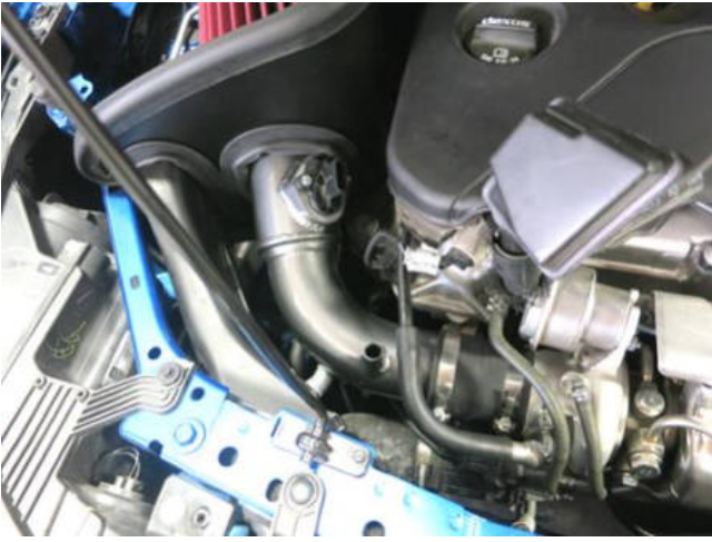
k. Adjust the tube orientation for best fit, ensuring the air filter does not contact any part of the vehicle, and torque the tube-side hose clamp to 30 in-lb.
