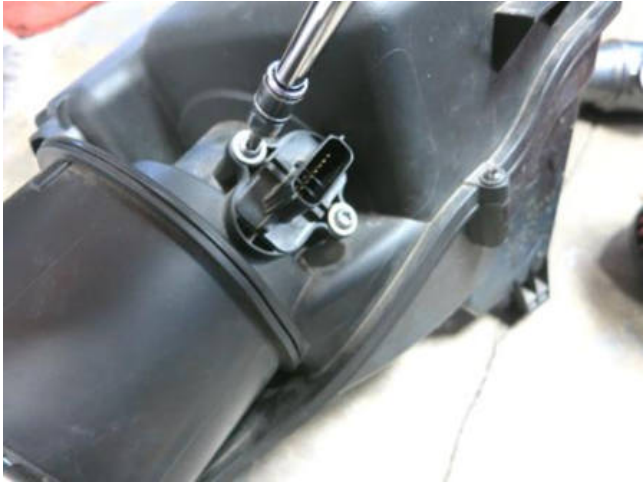
h. Using a T25 Torx bit, remove the MAF from the air box. These screws will not be reused. Note: Do not discard any of your stock equipment.
