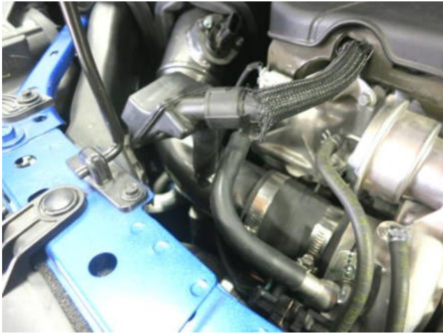
l. Install the PCV hose onto the intake tube.
