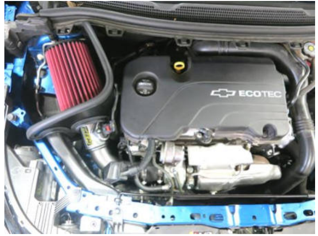
AEM INTAKE INSTALLED
