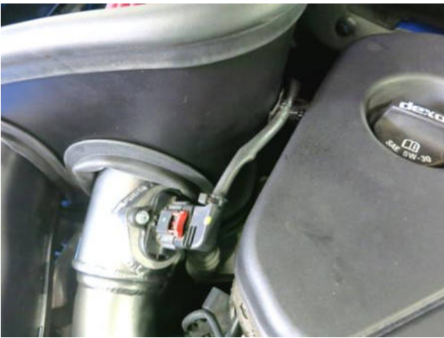
m. Connect the MAF harness and lock by sliding the red tab and clip the MAF harness wire tie to the heatshield.
