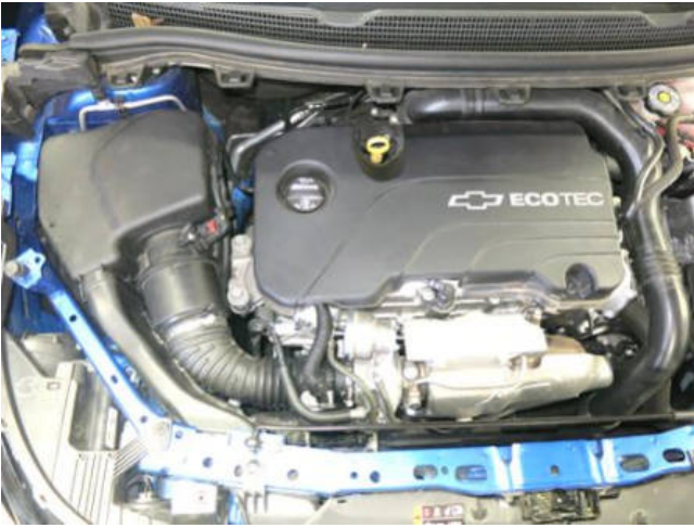
STOCK INTAKE INSTALLED
