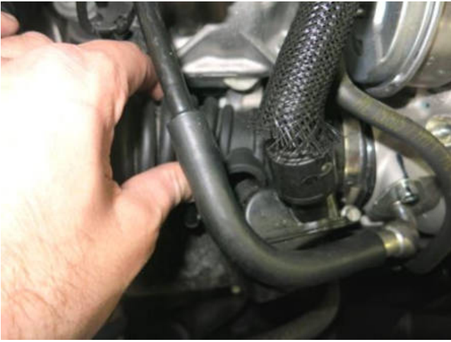
e. Gently disconnect the PCV reservoir by pinching the intake hose while pulling the reservoir free.
