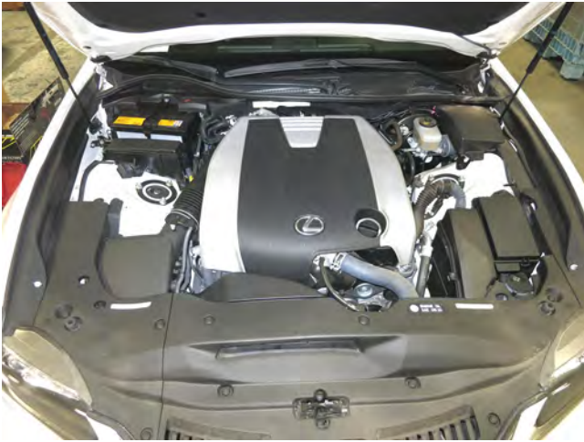
STOCK INTAKE INSTALLED
