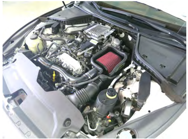
AEM INTAKE INSTALLED (ENGINE COVER REMOVED)
