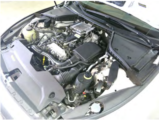
STOCK INTAKE INSTALLED (ENGINE COVER REMOVED)
