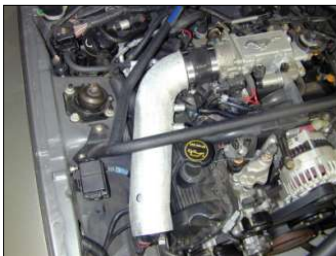
c. Insert inlet pipe into coupler. Do not completely tighten hose clamp.
