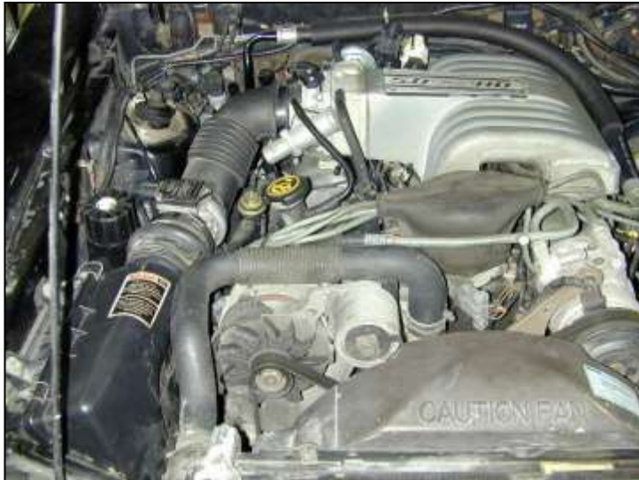
Factory air box system installed
