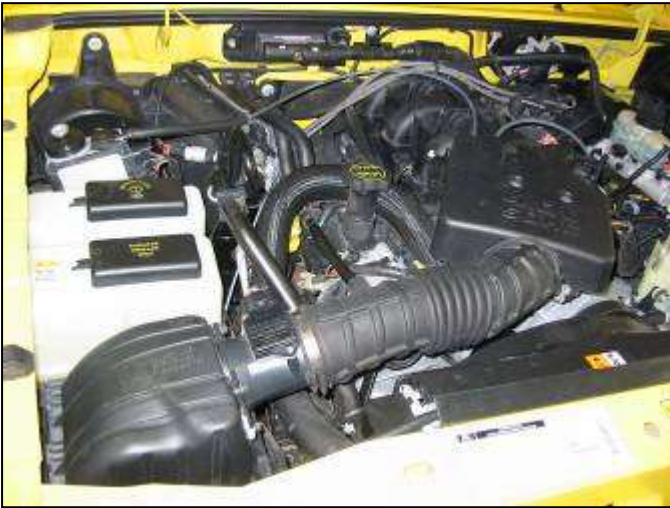
a. Factory air box system installed.
