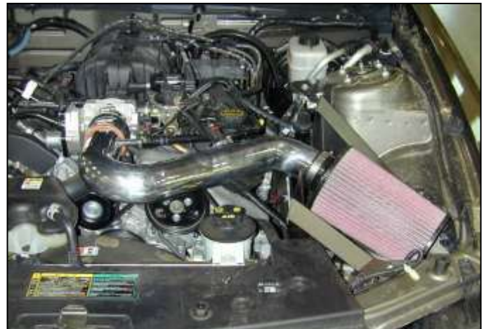
AEM® intake system installed
