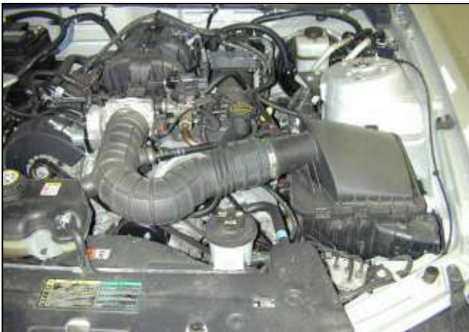
Factory air box system installed
