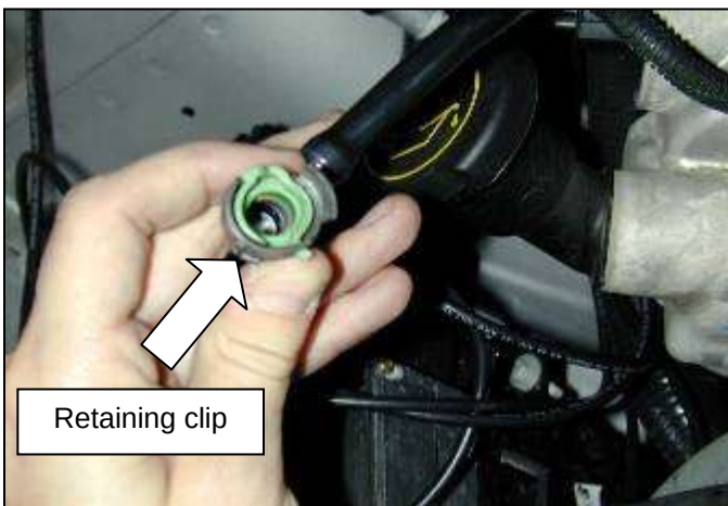
c. Loosen the hose clamp on the throttle body attached to the stock intake hose. Unplug the plastic breather hose connected to the intake hose. This is done by sliding the green retaining clip until the hose is free from the nipple.
