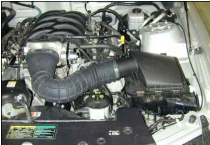
a. Factory air box system installed.
