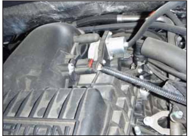
b. Locate the mass airflow sensor and the connector on the air box.
