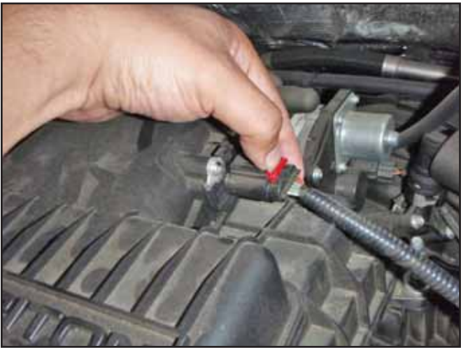
c. Release the locking mechanism on the connector.
