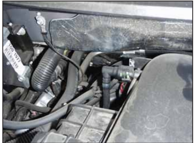
f. The PCV hose is located on the opposite side of the air box from the mass airflow sensor.
