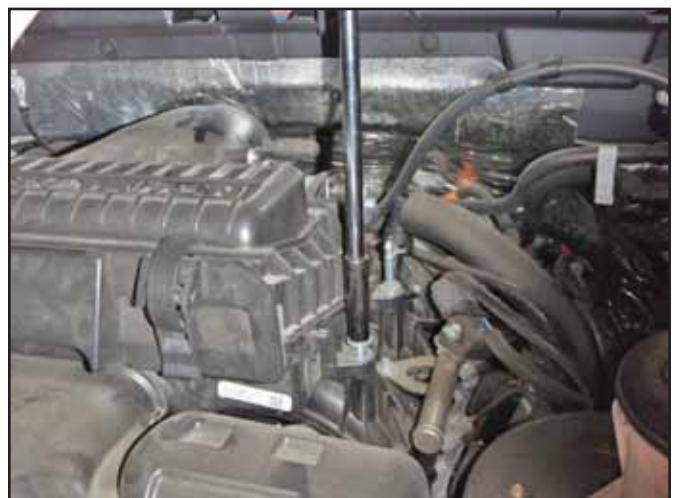
j. Remove the two bolts located on the driver side of the air box.
