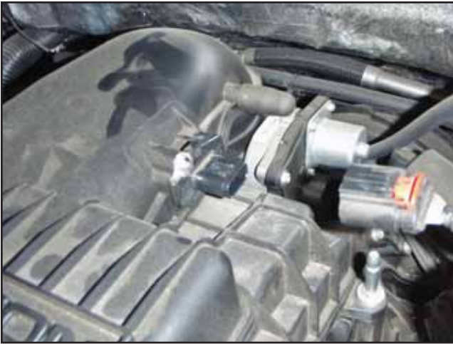
e. Connector disengaged from the sensor.
