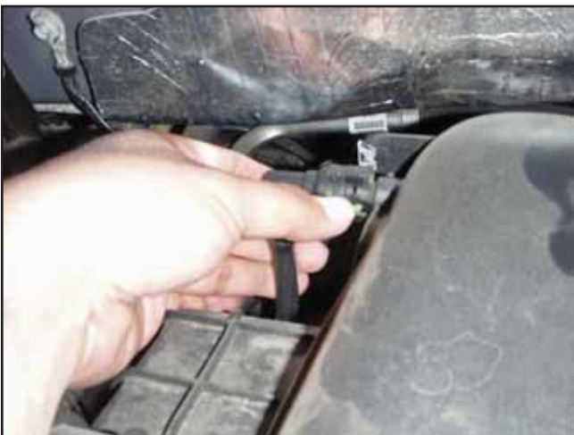
g. Release the green locking mechanism on the PCV hose connector.
