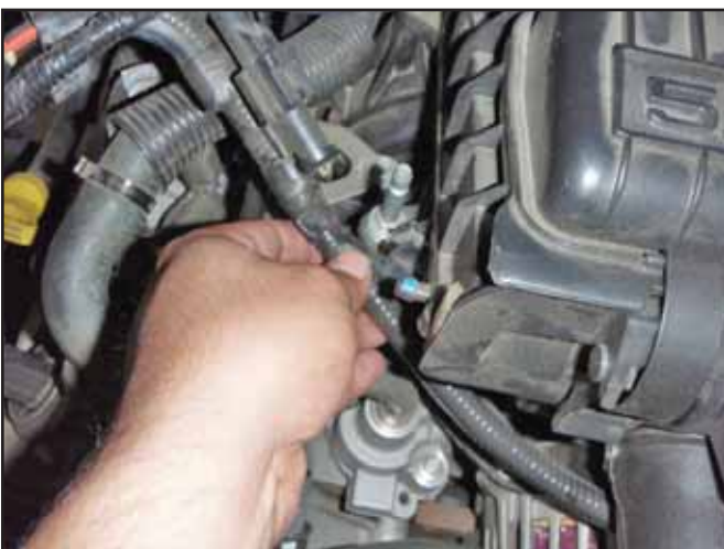
i. Unclip the wire harness attached to the air box located on the lower left hand side of the air box.
