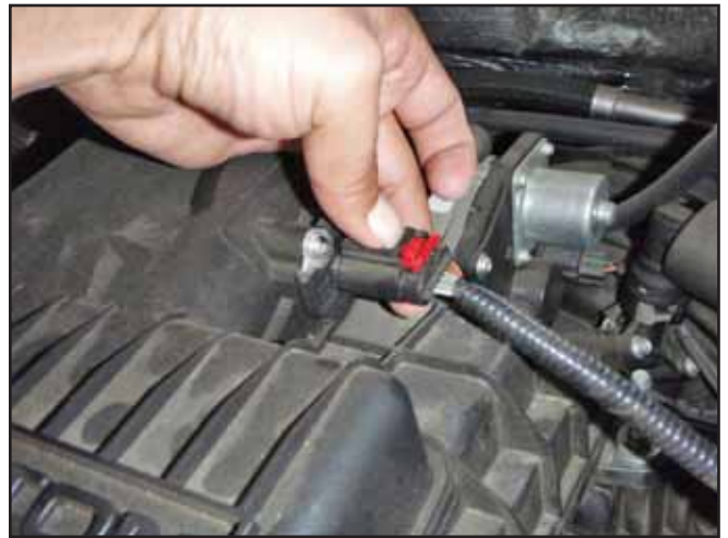
d. Press the plastic clip on the connector down and pull the connector away from the sensor.
