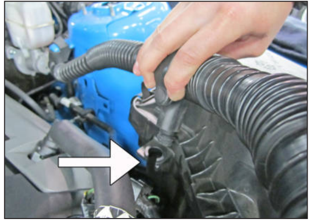
f. Lift up on the rubber support to release it from the OEM airbox.
