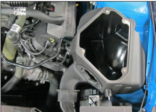
h. Lower the AEM® airbox into position as shown.
