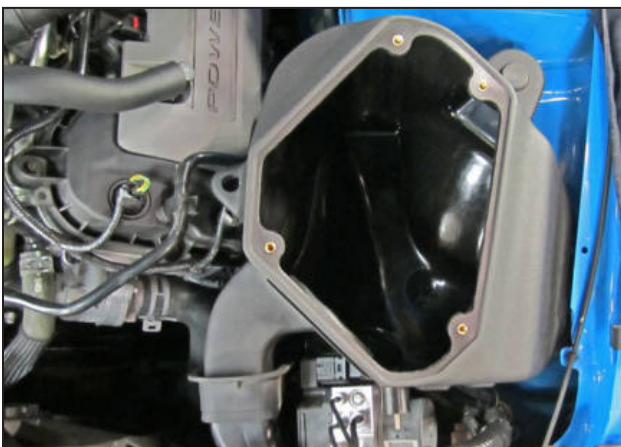
j. Guide the two bosses on the bottom of the AEM® air box into the grommets installed in step 3g.
