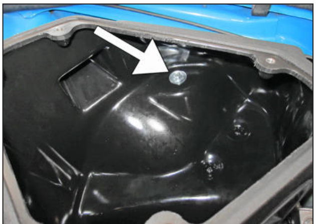
k. Secure the airbox to the vehicle's frame using the supplied M6 bolt (# 1-2038) and washer (# 08160).
