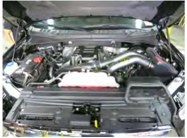
AEM INTAKE INSTALLED
