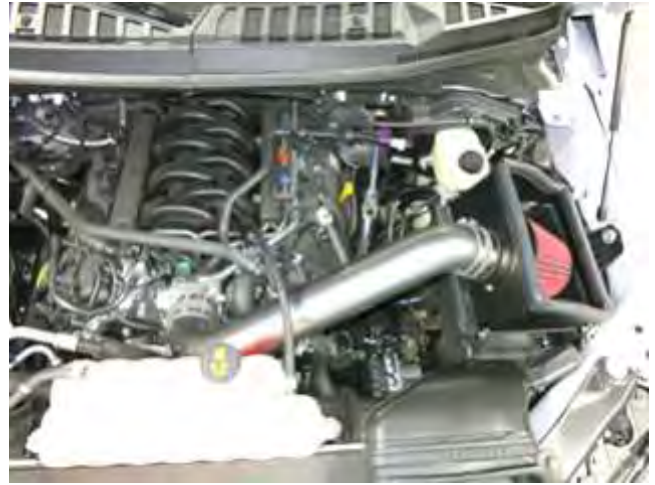
p. Finished installation of AEM Intake System.
