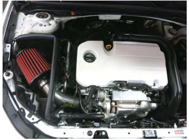
AEM INTAKE INSTALLED
