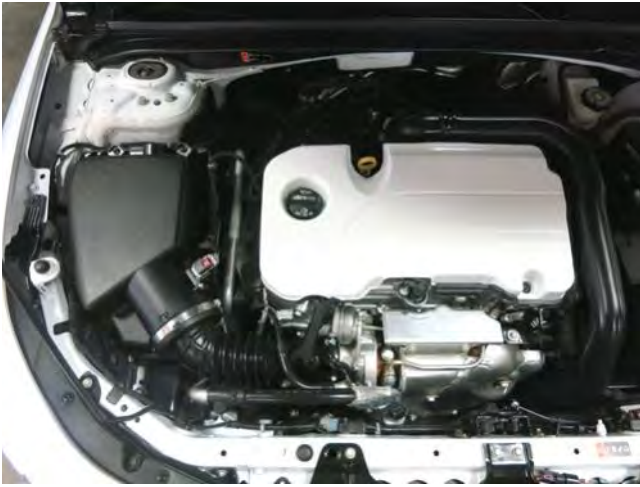
STOCK INTAKE INSTALLED
