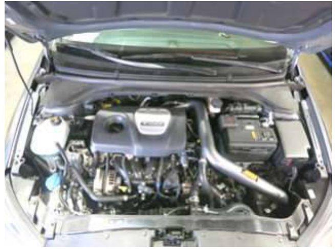
AEM INTAKE INSTALLED
