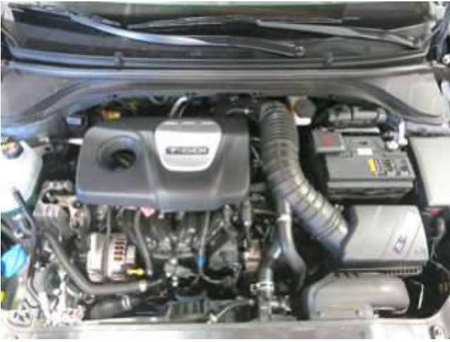
STOCK INTAKE INSTALLED
