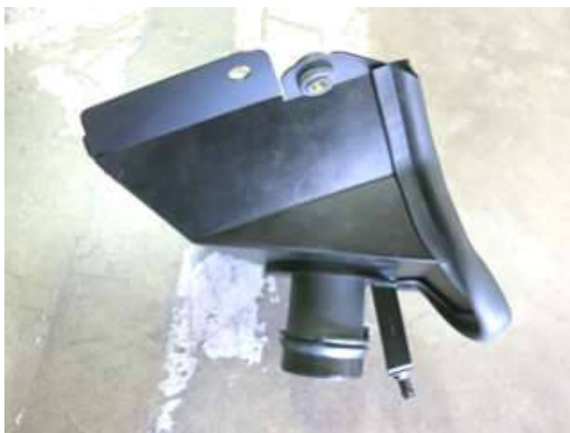
c. Assemble the driver side intake system as shown. Take care to use the correct MAF housing bracket (part number "7-363" will be stamped on).
