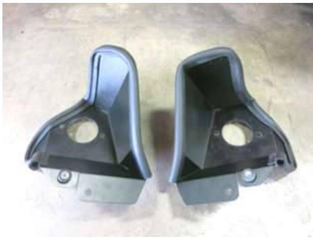
a. Apply edge trim to both heat shields as shown. Cut the single 80" length of trim as necessary. Also install the grommets and sleeves removed in step 2h.
