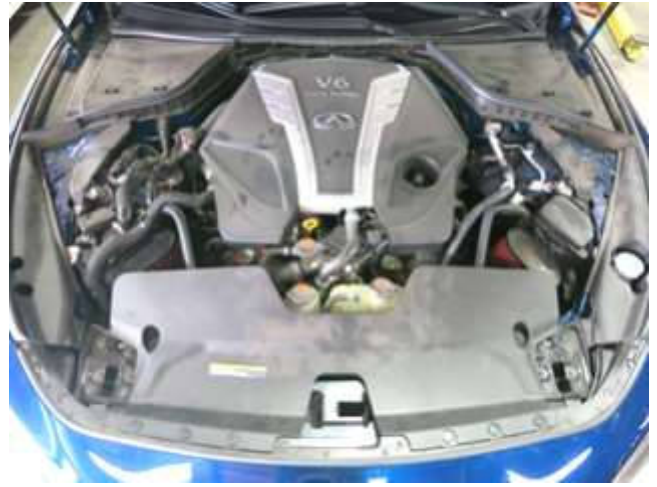
AEM INTAKE INSTALLED
