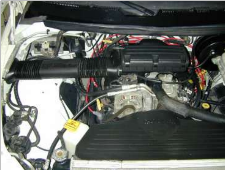
Factory air box system installed
