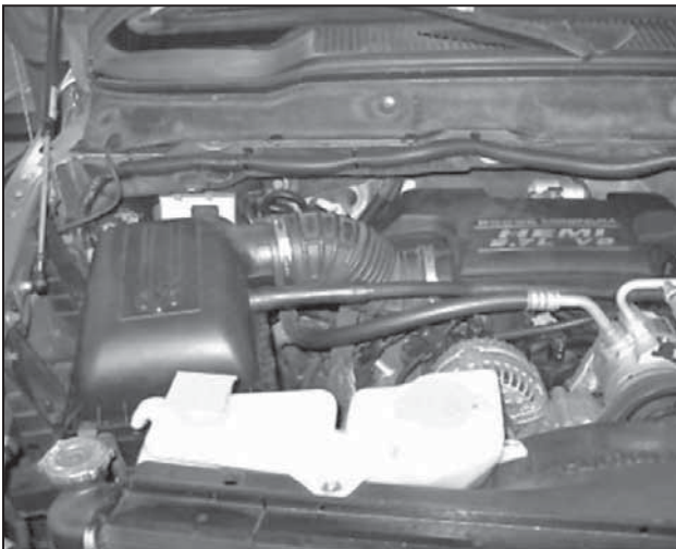
Factory airbox system installed
