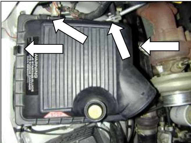
c. Release four clips and remove upper air box.
