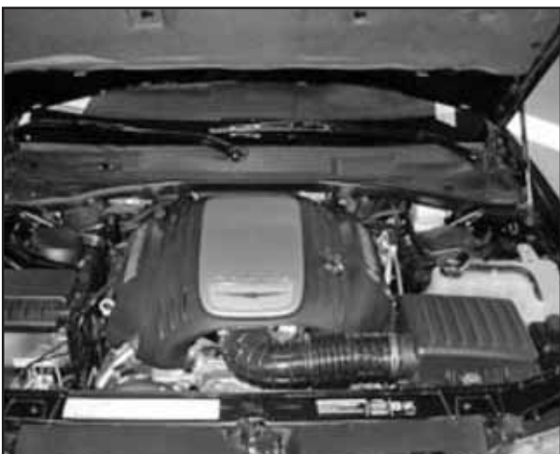
Factory air box system installed
