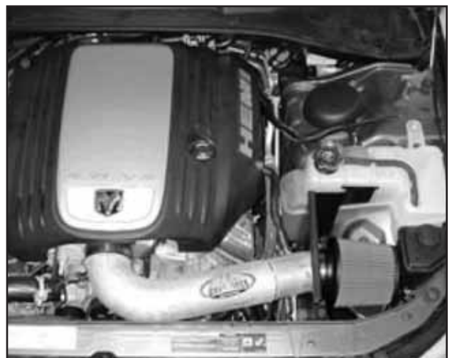
AEM® intake system installed
