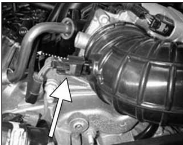
c. Pull out the locking clip for the intake air temperature (IAT) sensor.
