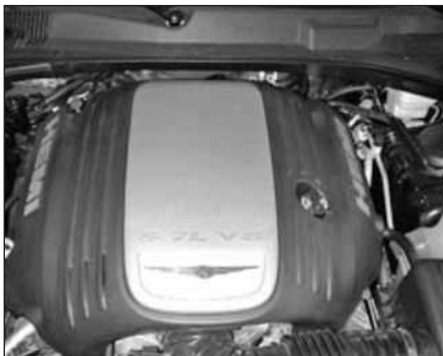
b. Remove the engine cover by pulling straight up.
