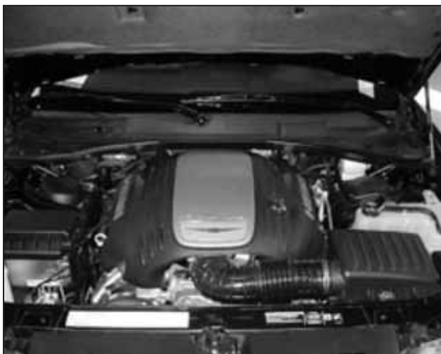
a. Factory air box system installed.
