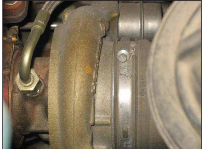
b. Loosen the hose clamps securing the flexible inlet hose between the turbo inlet and the air filter housing. Remove the inlet hose.
