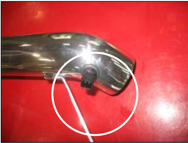
f. Insert the IAT sensor into the grommet from step 3c.
