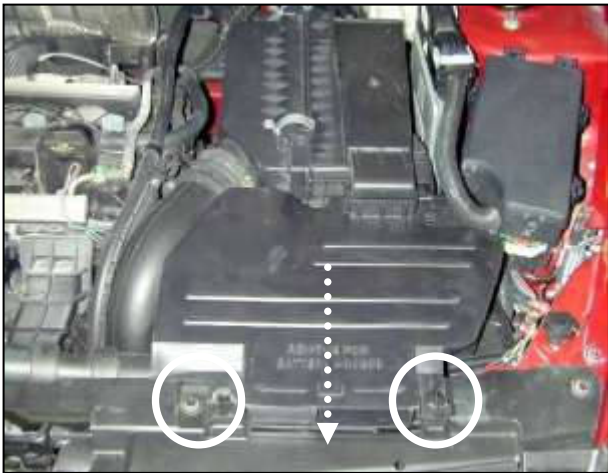
b. Twist and remove the retaining clips. Remove ducting by pulling up and forward.
