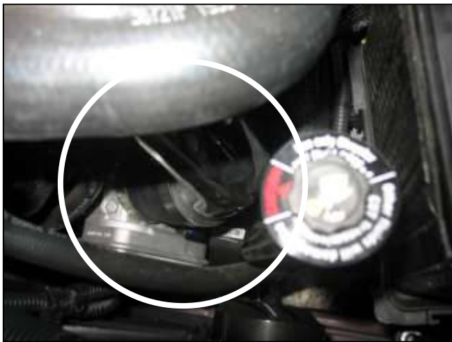
h. Insert the other end of the inlet pipe into the coupler at the throttle body. Realign the bracket and secure the hose clamp.
