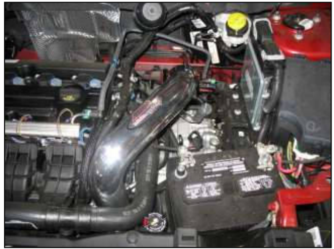
g. Insert the intake pipe as shown. Line up the pipe's bracket with the spacer assembly.
