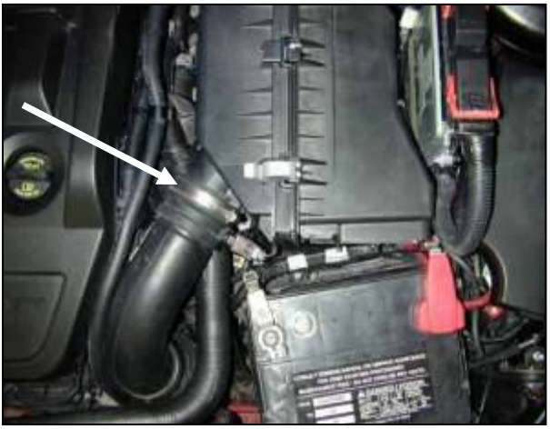
c. Loosen the hose clamp at the air box inlet.
