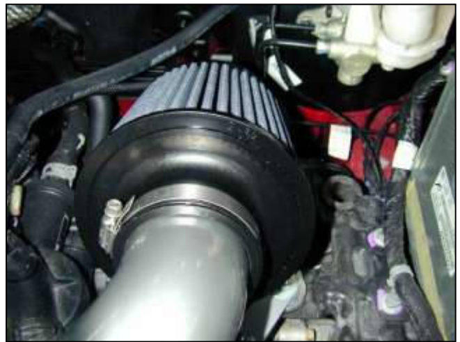
i. Attach the air filter. Check for clearance and secure hose clamp.
