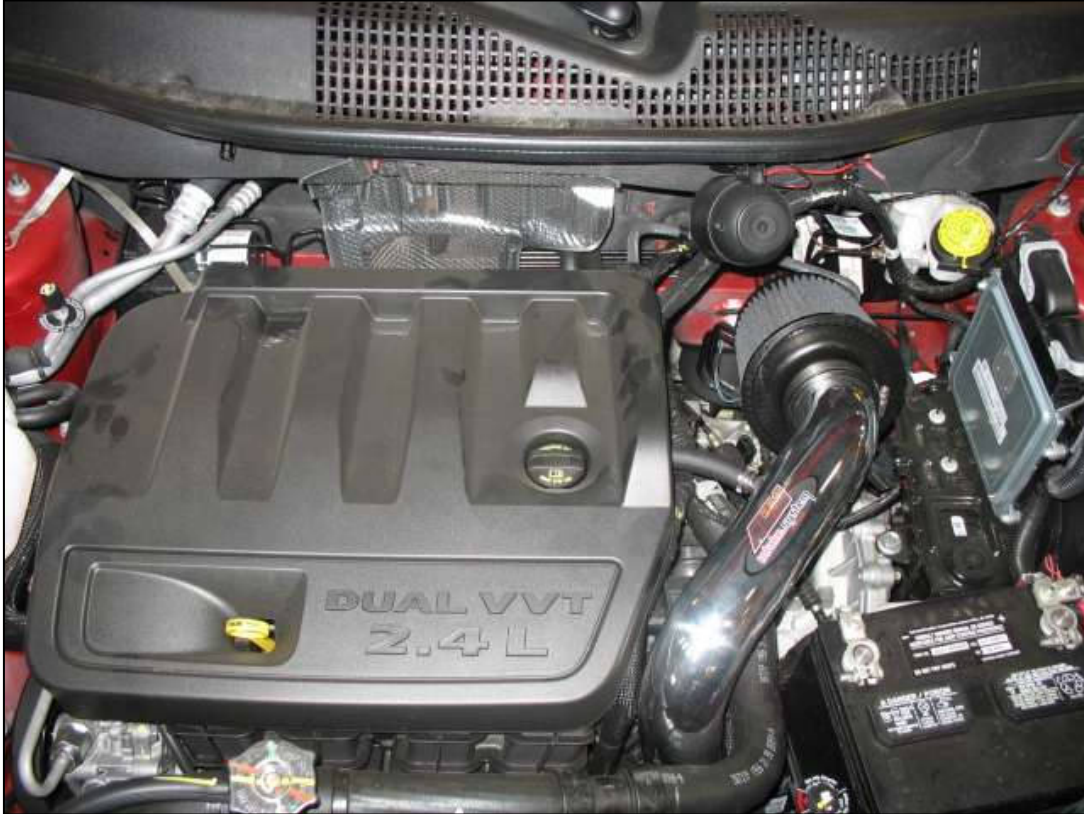
AEM® intake system installed
