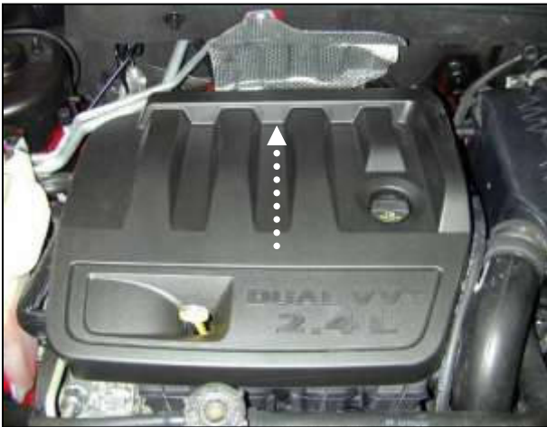
a. Remove the engine cover by pulling straight up.
